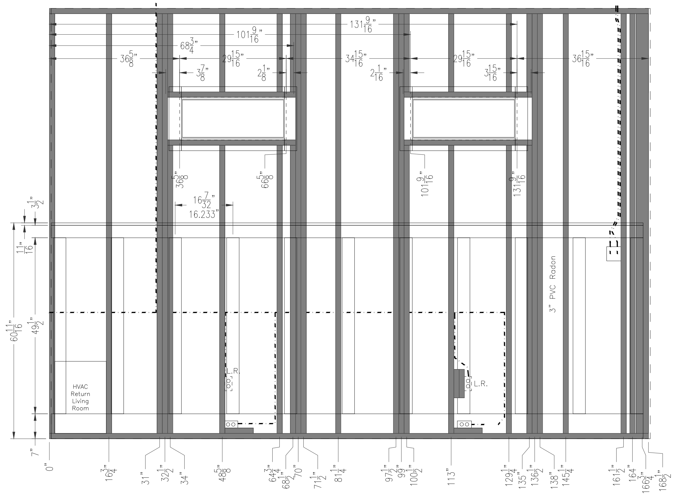
Dining Room - West Wall Stud & Wainscoting Location
